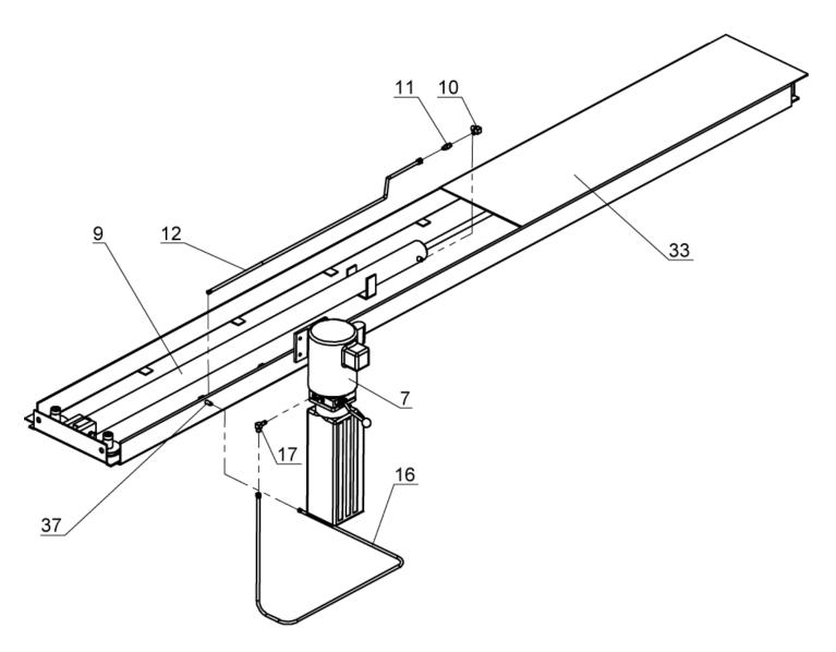
HYDRAULIC & CYLINDER COMPONENTS -  $\underline{\text{FIGURE \# 6}}$
